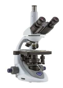
Trinocular brightfield microscope, 1000x, N-PLAN objectives
