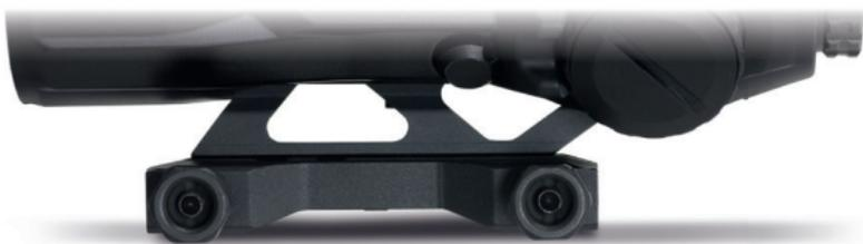
Once properly located on the rail, tighten the base nuts to 3.5 Nm. To further meet your needs, the sight height could be adjusted by installing one of the two included spacers (3 mm or 5 mm) which raise the height to 42 mm respectively 44 mm.
