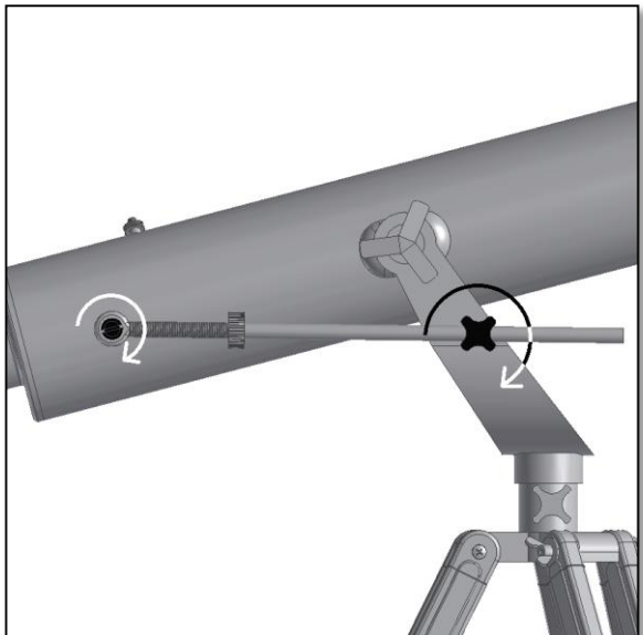
Figure 7. Fine focusing shaft in place.
