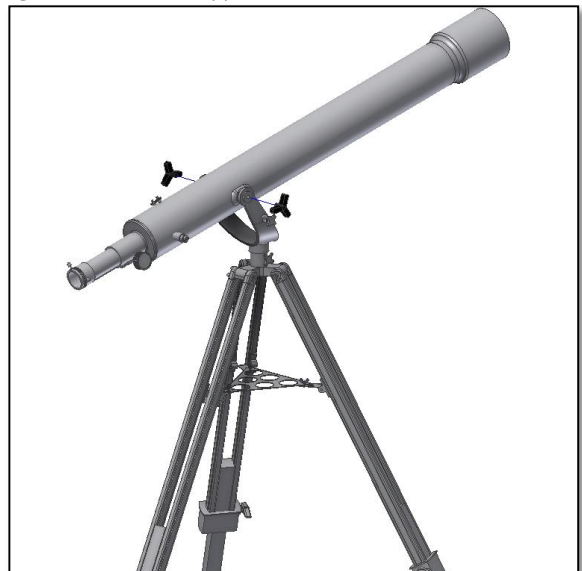
Figure 5. Insert the tube in the fork mount and fix it.
