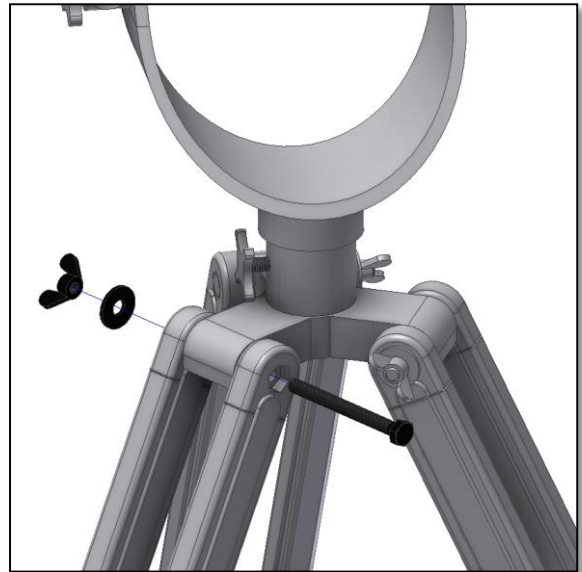
Figure 3. Insert the supplied screw, washer and nut.
