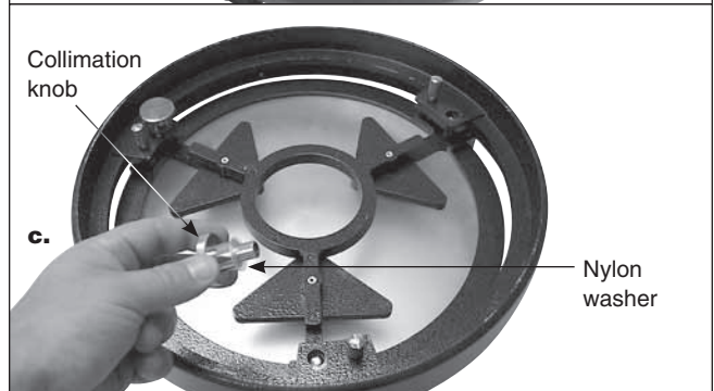
Figure 16. Shown for XX12g. a) Place the three springs on the exposed threaded shafts of the mirror cell. b) Lower the rear end ring onto the mirror cell so that the threaded shafts pass through the end ring, and the end ring rests on the springs. c) Thread the collimation knobs, with nylon washers attached, through the rear end ring and onto the threaded shafts. Make sure the knobs have at least three full turns of engagement on the shafts.
