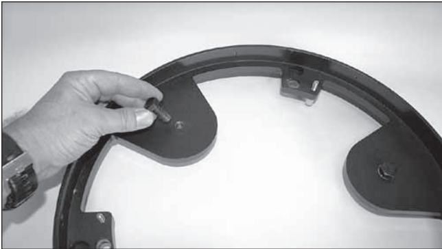
Figure 15. Thread the three hex-head counterweight mounting bolts (XX14g and XX16g only) into the holes in the counterweight support plates as shown. Tighten using an adjustable or 16mm crescent wrench.
