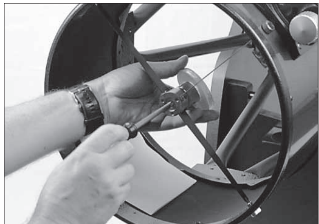
Figure 30. To center the secondary mirror under the focuser, hold the mirror holder in place with one hand while adjusting the center bolt with a Phillips screwdriver. Do not touch the mirror's surface!
