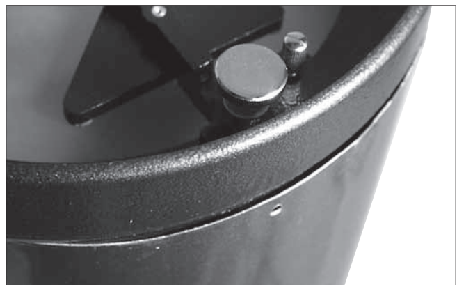
Figure 17. Locate the area of tube that is bulging out and preventing the end ring from fully seating. Press on this bulge to allow the mirror cell to seat properly on the tube. Be careful not to pinch fingers!
