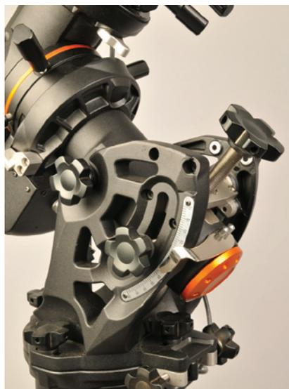
**A large hand knob and built-in latitude scale make it easy to set the mount's polar-axis elevation. Fine threads on the adjustment screw aid in precise tweaking of the elevation during polar alignment. There's a similar fine-motion adjustment for setting the mount's azimuth position.**
