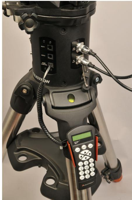
Most of the mount's electronics are housed in this 6-inch-diameter pier column. Cables for the drive motors, as well as the one for the external 12-volt DC power supply, use threaded connectors that prevent the cables from being accidentally pulled loose during use.
