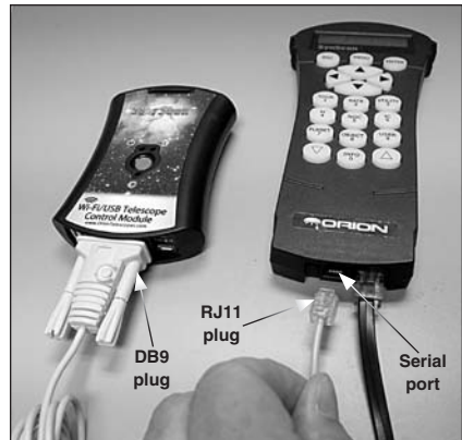
Figure 4. Connecting the StarSeek module to the SynScan hand controller. The RJ11 plug on the serial cable connects to the serial port on the SynScan, which is right next to the larger RJ45 port for the coil cable.
