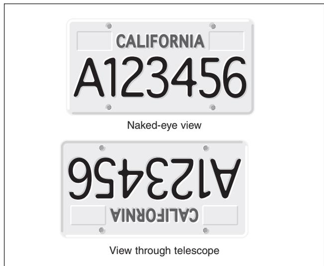
**Figure 16.** The view through a reflector telescope is upside down. This is true for the SkyQuest XT IntelliScope.
