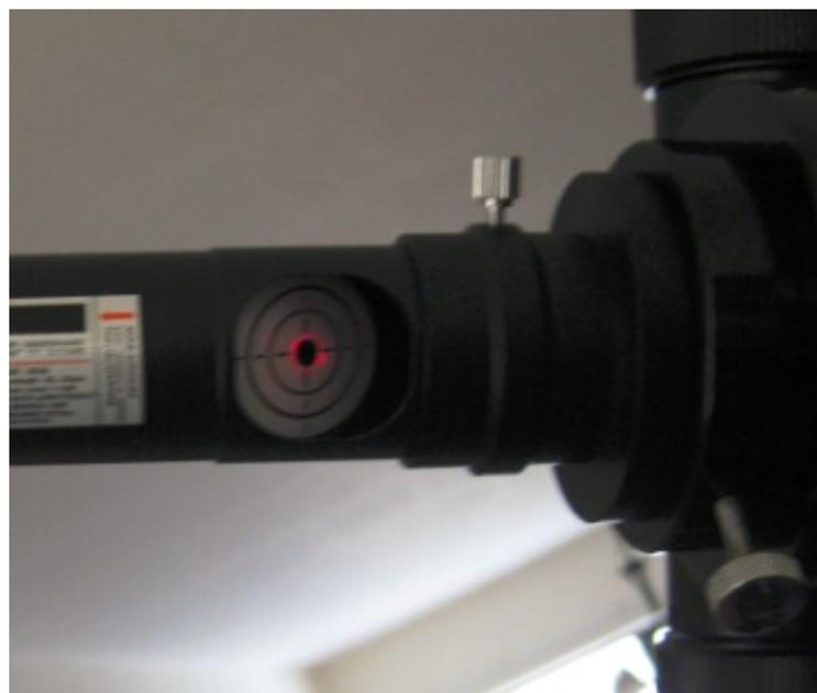
**Figure 6: The primary mirror is perfectly collimated by laser collimator.**
