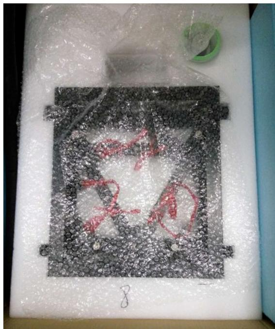
The Mirror Box Protection Ring is bolted to the mirror box by the knobs. The secondary mirror safe container is at the up right corner in the above picture. The protection ring is not used to assemble the scope, and is only used to pack the scope.
