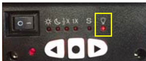
Figure 22 Polar scope LED intensity adjustment
