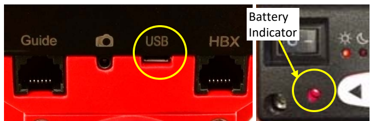
Figure 8. Micro USB powering/charging port
