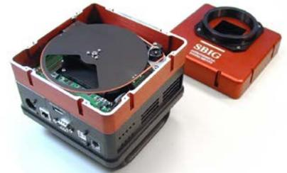
3. Attach the filter wheel base to the red spacer that is attached to the camera body. At this point you should install the filters if not already installed.
