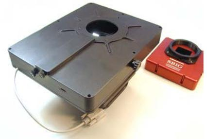
5. Both the FW8S-STXL and FW8G-STXL filter wheels have this "pig tail" cable with a DB9 connector on the end. Plug this connector into the I<sup>2</sup>C port on the camera. .
