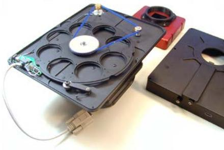
4. Replace the filter wheel front cover being careful not to pinch the cable that extends from one end.
