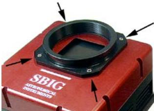
7. Finally, remove the 3" adapter ring from the camera front cover being careful to note the location of any shims used to assure orthogonal camera position and attach this adapter plate to the front cover of the filter wheel replacing the shims, if any, in the same locations.
