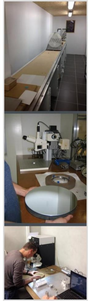
Our workshop is equipped with a test bench of 6 meters long mounted on anti-vibration isolators.
