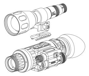
FIGURE 2-8. MOUNTING AN IR ILLUMINATOR
