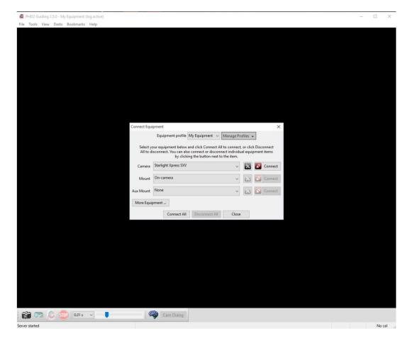
Next, press the 'Mount' button and select 'On camera' (this uses the RJ12 cable to feed corrections to the mount). You can also set these as the default by using the 'Manage Profiles' selection at the top of the box. Close the settings window when finished.
