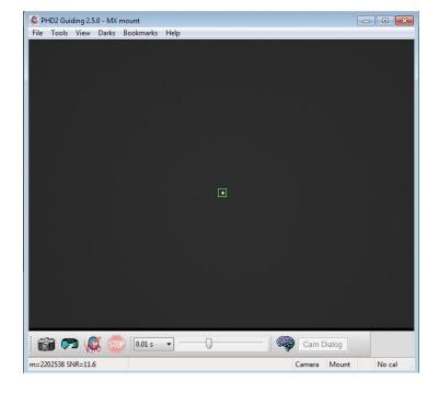
Click the mouse on a suitable guide star in your last image and then select the 'Target' icon. PHD2 will set up a cursor and box on the guide star and proceed to 'calibrate' the mount. After about 1 minute of calibration, it will start to guide on the star.
