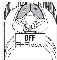
You can deactivate the SWAROLIGHT function by turning the OFF/DAY/NIGHT switch to the central position and pressing the +/- buttons at the same time for 6 seconds. The light will flash twice to confirm that the function is deactivated. You can reactivate the SWAROLIGHT by repeating this step.
