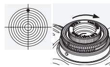
Turn the outer knurled ring on the top turret in the opposite direction to H (clockwise).
