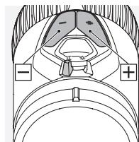
the ideal level of brightness quickly, you can press and hold one of the buttons (long pulse). To make precision adjustments, press either of the buttons once (single pulse).
