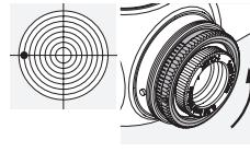
Turn the outer knurled ring on the side turret in the direction of R (counter-clockwise).
