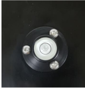
Figure 18. Bubble level for AA mount leveling
