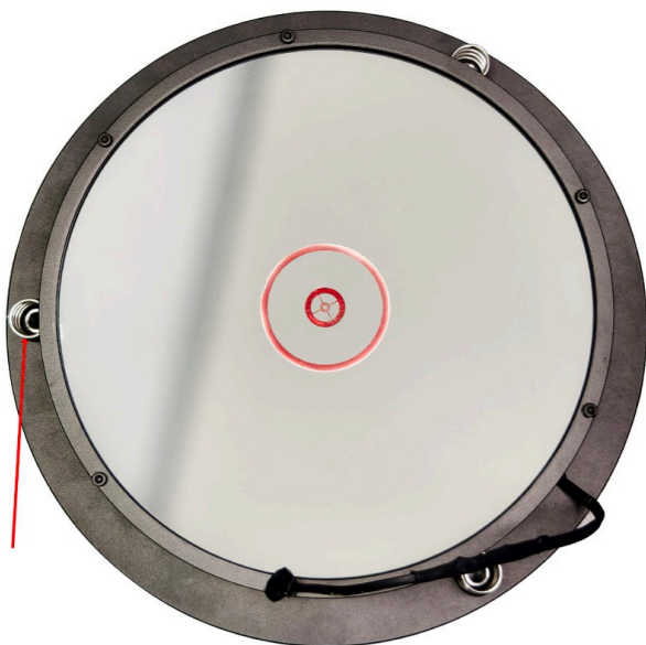
Figure 1: Place the bracket for the main mirror on a flat surface. Lay the power cable for the main mirror heater over the top of the mirror and ensure that it remains inside the bracket. Insert three springs into the recesses provided.
