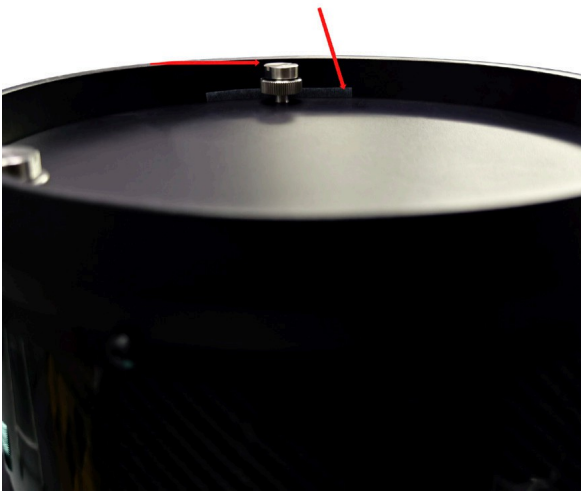
Figure 6: The final position of the mirror mounting screws should be below the edge of the mirror base so that the three exposed rubber limiting strips are clearly visible.
